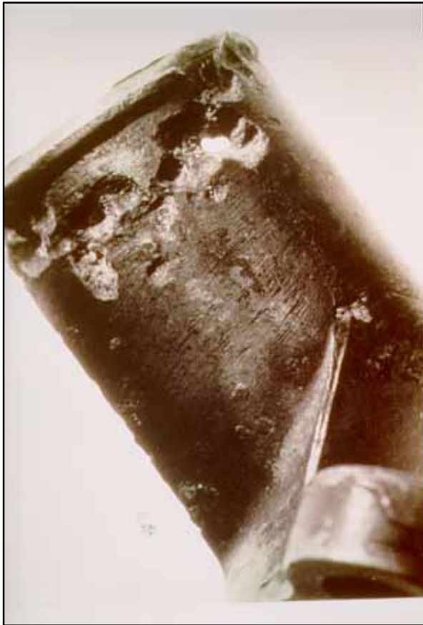
Severe crevice attack of coolant outlet
