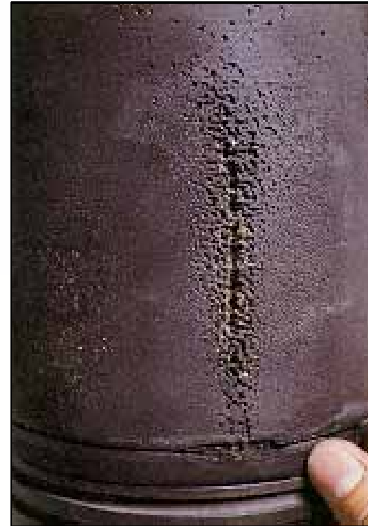
Cooling System Liner/Water Pump Pitting, TF-158, Nalco
