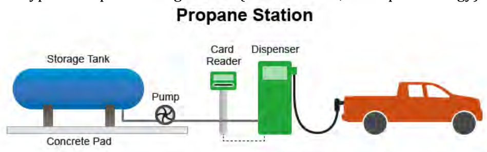
Figure 3. A Typical Propane Filling Station (Source: AFDC, US Dept of Energy)
